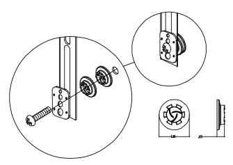
The universal spacer may be stacked five (5) high, for a total stacking height of 1-1/4". The universal spacers must be stacked in the direction shown above. The universal spacers must be placed between the mounting bracket and the flat-panel. The universal spacer can fit M4, M5, M6 and M8 screws sizes.
