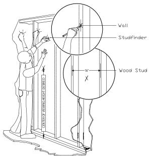
**Step 1.** Using a (commercially available) wood stud finder, locate the 16" or 24" stud centers behind the wall.
