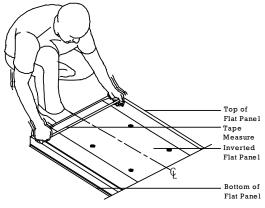
**Step 1.** Once the flat panel is inverted, use a measuring tape to find the center of your flat panel measuring from outside to outside of the chassis.
