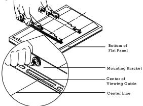
**Step 4.** The mounting brackets are designed with a center viewing guide on the side.
