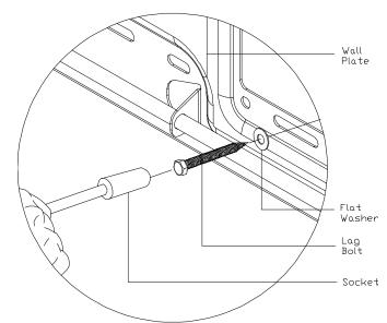
**Step 6.** Secure the plate using the four (4) 5/16" lag bolts and flat washers.
