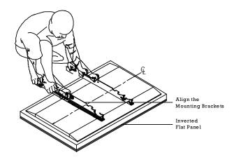
**Step 3.** Match the center of viewing guide with the center line you marked in step 1.
