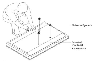
**Step 1.** Place the universal spacers over the mounting points on the flat panel.
