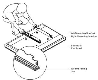
**Step 2.** Lay the mounting brackets (stamped arrows facing out) on the display, over the mounting points.
